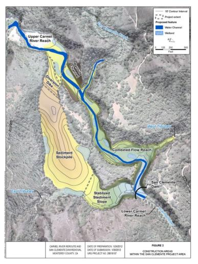
Figure 34. Design plans for rerouting the Carmel River and sediment stockpiling and stabilization for the CRRDR alternative (figure courtesy of San Clemente Dam Removal and Carmel River Restoration, all rights reserved).
