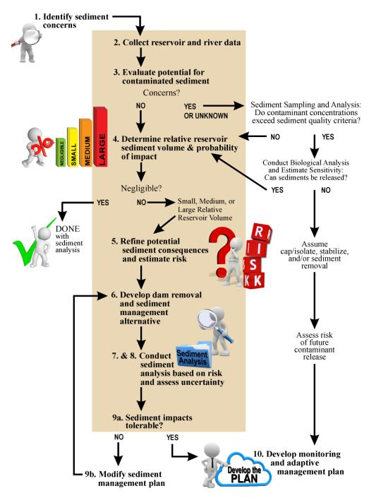
Figure 16. Sediment analysis steps for dam removal (Randle and Bountry 2017).
