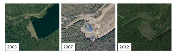
Figure 26. Aerial photographs of Birch Run Dam before, soon after, and 5 years after dam breaching.
